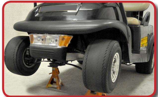
Detach front bumper by removing the two factory bolts closest to the edge of the frame. Retain bumper and hardware.
