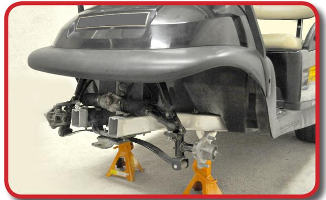
Using a 21mm Socket remove and retain hub and flange nut. Repeat on passenger side.
