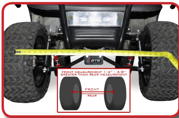
Ensure the wheels are pointing straight forward. To adjust Toe, find a common point to measure from on the inside front and inside rear of the front tires. Adjust until the front measurement is 1/4" to 3/8" greater than the rear measurement.
