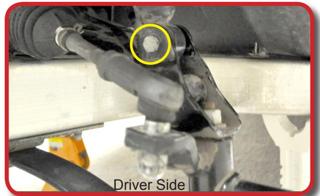
Remove and retain the cotter pin from the tie rod end, using an 18mm Socket and an 11/16" Wrench. Remove nut from tie rod.
