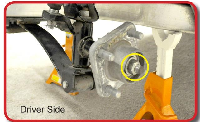
Using a 1/2" Socket remove bolt from shock and discard push shock up and out of the way.
